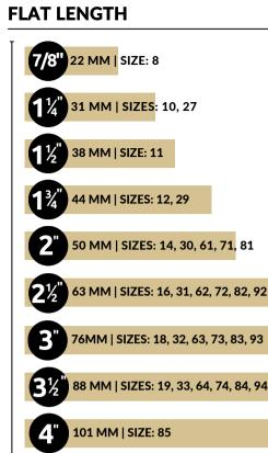
Rubber bands have three core measurements that communicate their dimensions: flat length, band width, and lay the band flat. The distance from end to end is the flat length. Perpendicular to the length is the band width. The wall thickness measures the thickness of the band.
